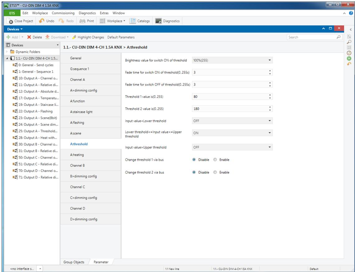
Fig. 4.4: “Threshold” window
