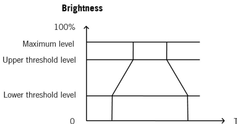
**Fig. 2.5:** Switch ON/OFF or Absolute dimming
