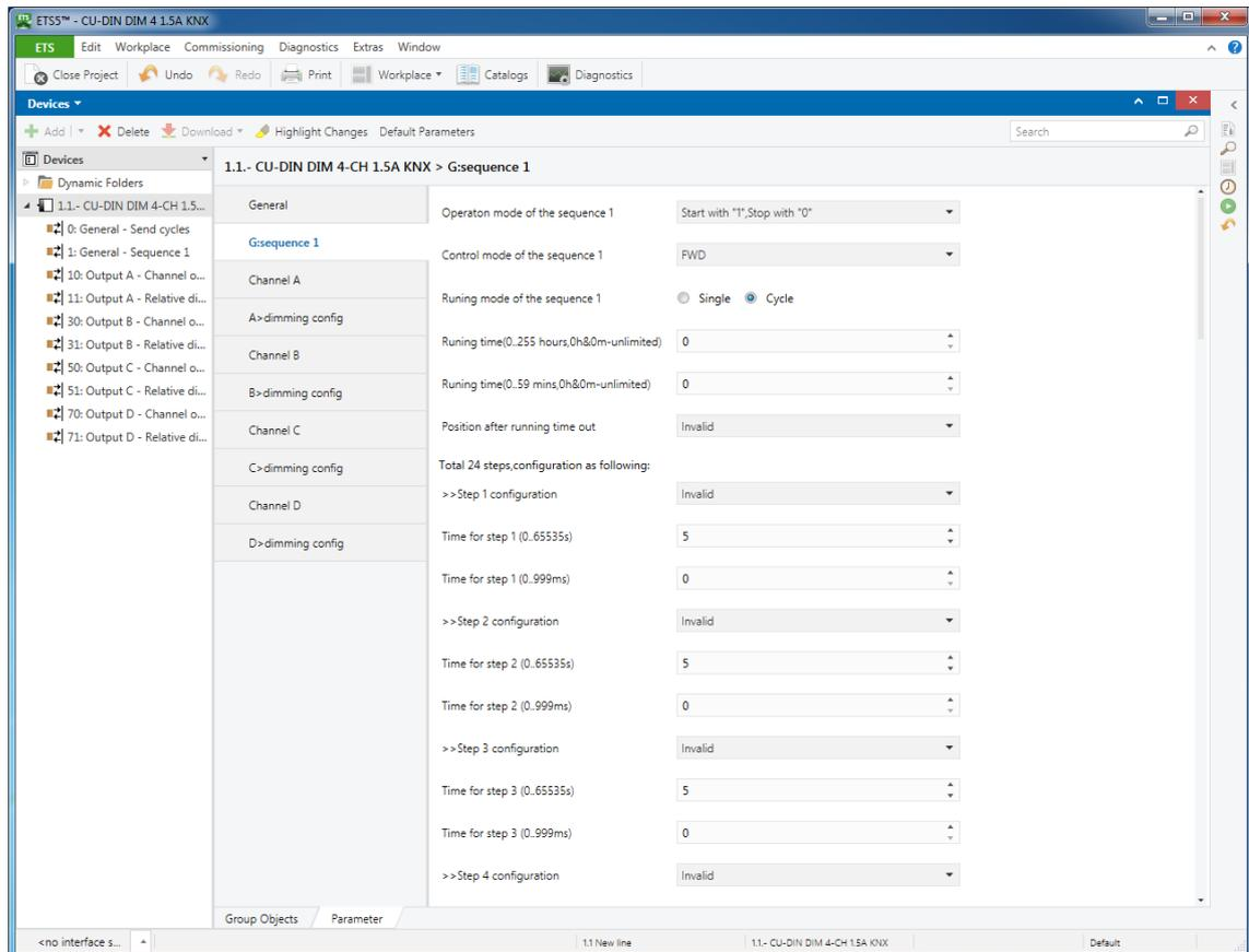
Fig. 1.1: “G: sequence 1” parameter window. This includes 24 steps.
