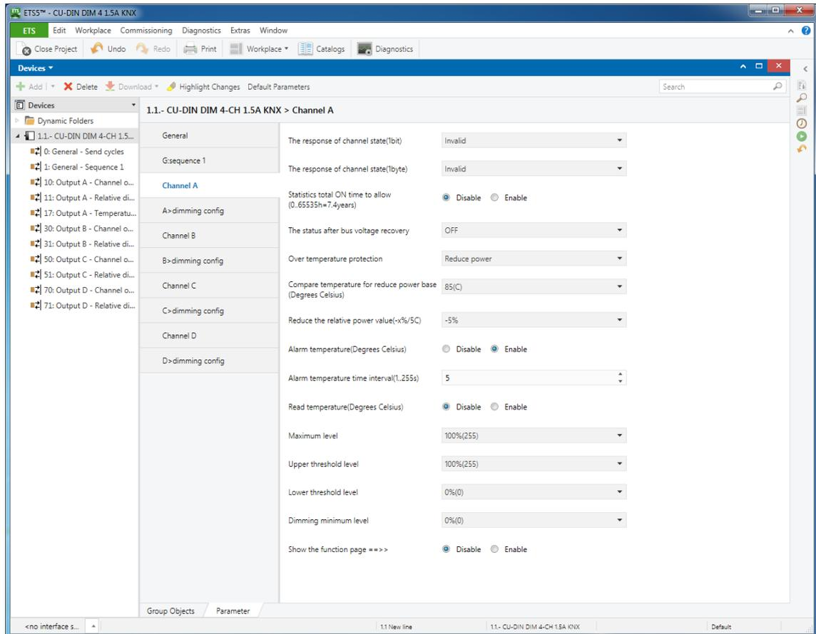
**Fig. 2.4:** “Over-temperature protection”
