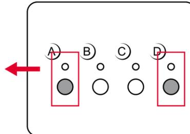
**Note:** Press and hold the first and last buttons simultaneously to toggle between leading edge dimming mode and trailing edge dimming mode.
