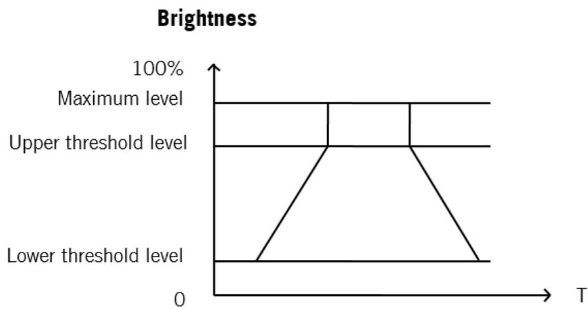
**Fig 2.6:** Relative dimming
