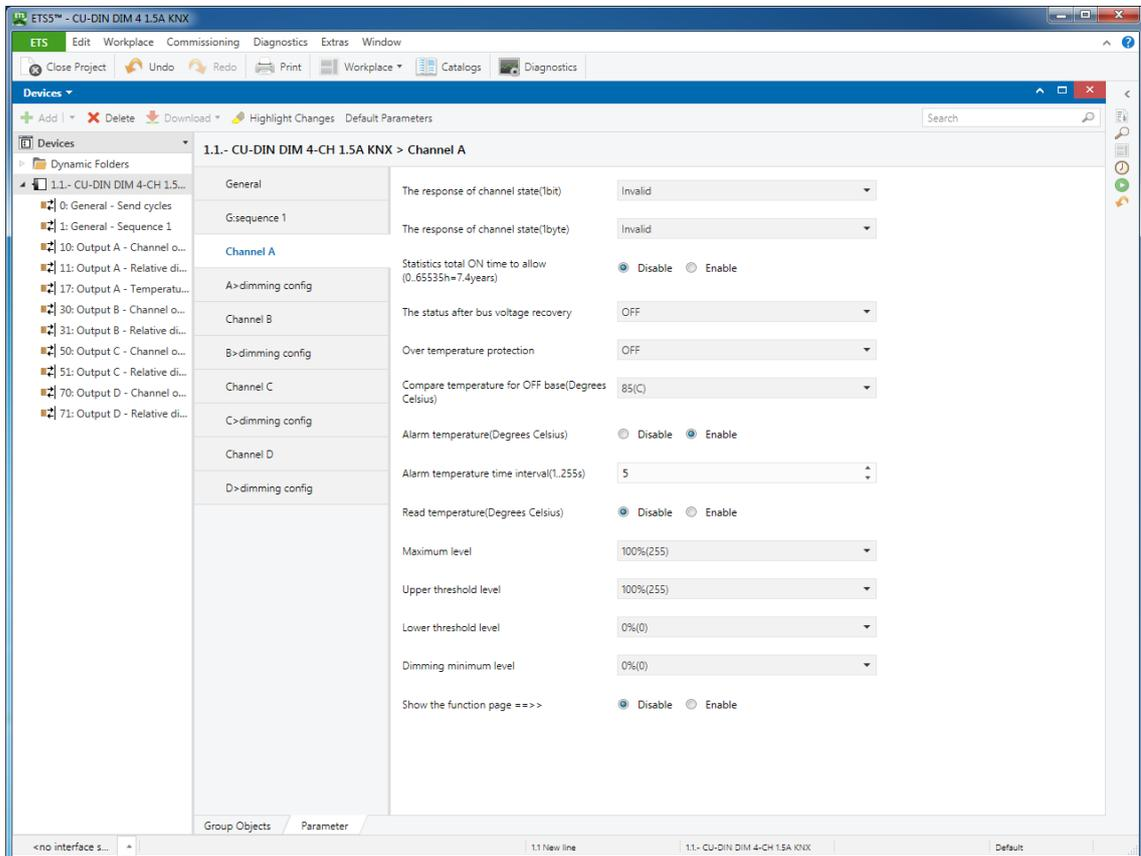
**Fig. 2.3:** “Over-temperature protection”
