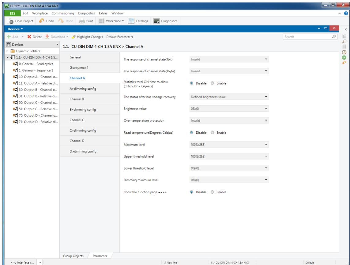
**Fig. 2.2:** “Status after bus voltage recovery”
